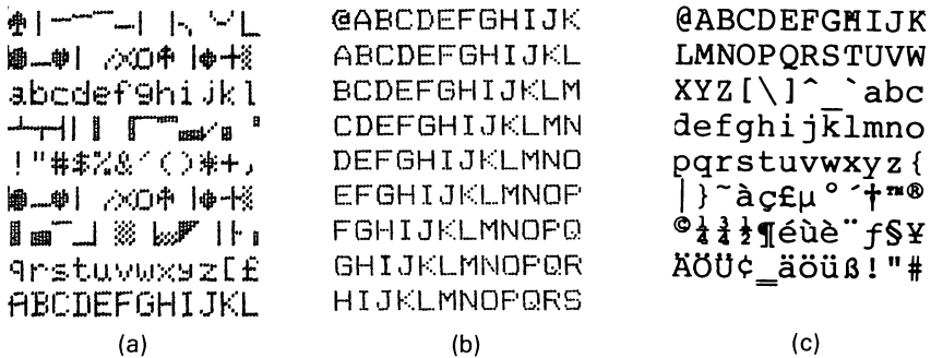
Fig. 1.2. Three samples of print from three different qualities of printer: (a) the Seikosha Vic printer, (b) the Epson FX80 printer and (c) the Tandy Daisy Wheel II printer.
