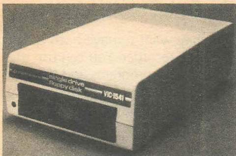
Commodore disk drive, to be used with diskettes for the VIC and 64.
